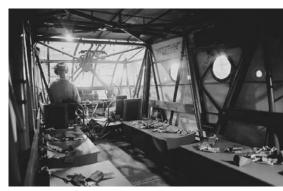
Fabric sides, no engine! Interior of WACO CG4-A glider configured for 13 troops. Typically towed by C-47, the 'Hadrian' could alternatively hold a jeep, a quarter ton truck, or a 75mm howitzer loaded through upswing nose section. 15 companies produced total of 12,000. *-Brian Mahoney*
