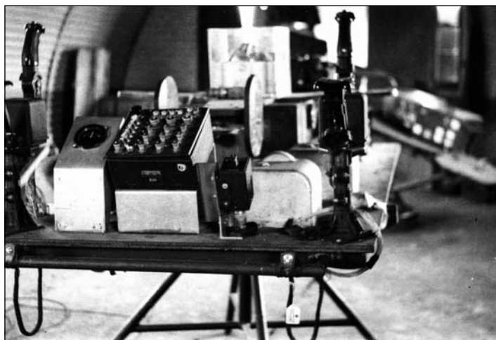
Part of Wayne Allen's rig for training on the C-1 and formation stick. Compare the sticks on left and right side of the table with the illustration of the formation stick in Herald #41. Armrest is clearly visible on right stick. In the center of the photo appears to be mock-up of vertical stabilizers. The rest of the C-1 table is visible in the background of this photo.
