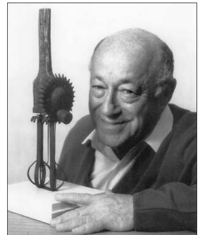
In order to give some chance of "lump-free" powdered eggs cooked in the POW camp, Ira fabricated this eggbeater from a slat from his bed and a sardine can, melting down the rivets to attach the handle. A great invention for Mother Necessity.
