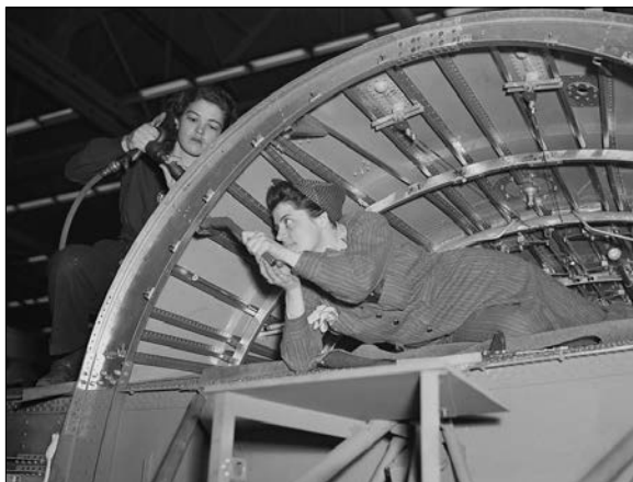
Here's the slightly dated original caption verbiage that ran with this photo when first released: "A girl team working on a center wing section of a B-24E (Liberator) bomber in Ford's big Willow Run plant. The Liberator is capable of operation at high altitudes and over great ranges on precision bombing missions. It has proved itself an excellent performer in the Pacific, in Northern Africa, Europe and the Aleutians. Ford's Willow Run Plant, Michigan." Photo: Howard Hollem/US Office of War Information, via Library of Congress.
