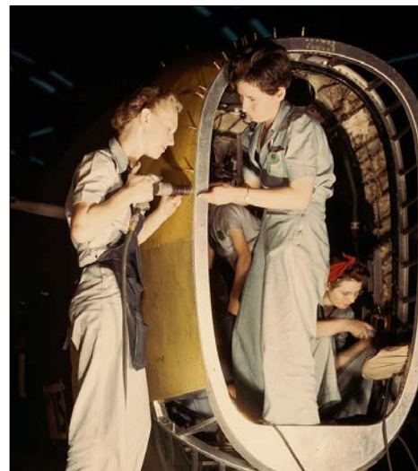
Liberator was designed to be manufactured in modules such as this, just ahead of the tail turret, that allowed rapid, intense fabrication detail and complexity by dispersing it. Work shown would have been much constrained if it were mated to neighboring fuselage segment any earlier than necessary. Photo: Howard Hollem/US Office of War Information, via Library of Congress.
