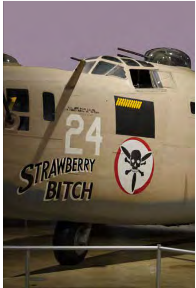
USAF Museum Liberator showing off its pilot-side pitot tube projecting into the air stream above where the number 24 appears. This model B-24 has a matching pitot tube on the copilot side. Photo: Pete O'Tube..
