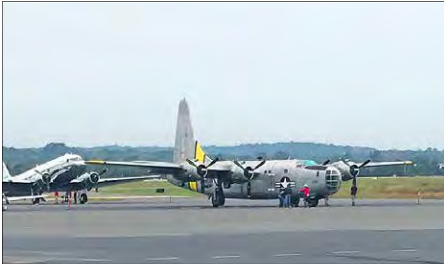
A flyable B-24 version parked on the ramp for the National Capital flyover. This is the PB4Y-2, one of two in flyable condition, which flew patrol for the Navy (note the straight tail). Longer and more stable than the B-24, it carried mines and bombs. Over 700 were built by Ford Motor. Photo: Chris Clark.
