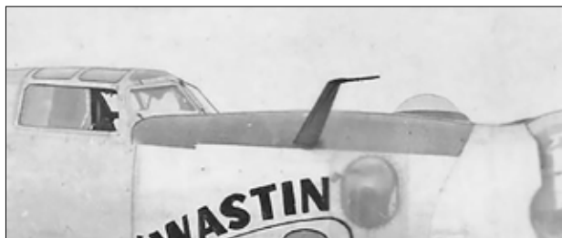
The pitot tube at the end of a prominent boom extension on the B-24. Located on both pilot and copilot sides of our beloved bomber to supply each pilot with independent readings, this device incorporated both the high and low pressure metering functions in each assembly. AAF photo.
