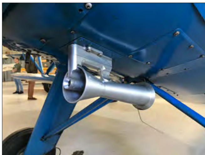
A substantial piece of milled aluminum. Located on underside centerline of beloved Waco workhorse trainer/liaison biplane, this late 1930s device was among earliest to incorporate both the high and low pressure metering functions in one assembly. From the Collings collection, American Heritage Museum. Photo: B. Mahoney.
