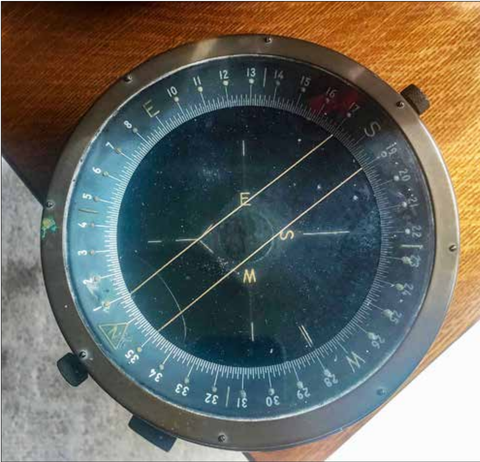
The US Army Air force Type-12 direct reading compass was used at the navigator's station on the nav-table of the aircraft. It was a key tool used by the navigator on B-17, B-24, B-29 and transports including C-46, C-47 and C-54. Photo: Freedom Museum.
